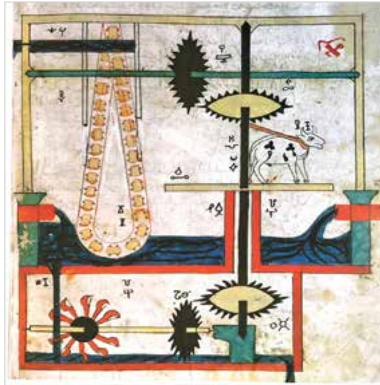
Figure 1. Water-pumping system from al-Jazzari, The book of knowledge of ingenious mechanical devices (1206)
